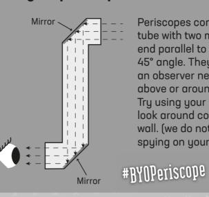
Periscopes consist of an outer tube with two mirrors at either end parallel to each other at a 45° angle. They are used when an observer needs to see above or around an obstacle. Try using your periscope to look around corners or over a wall. (we do not condone spying on your neighbours!)
